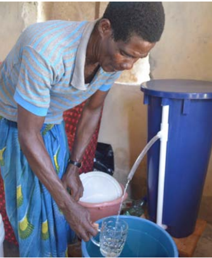
NDPI’s Appropriate Technology Enabled Development (ATED) program introduces simple, new technological solutions for development challenges in the region, such as the bio-sand filter shown above, which is a low-cost means of producing safe drinking water for households.
